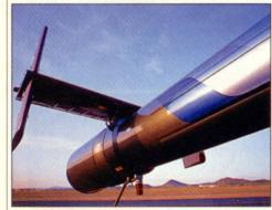
Air enters an intake behind the rotor mast and is compressed and forced into the tailboom by a high-speed fan. It exits through a pair of fixed slots in the right side of the boom, producing Coanda Effect, and through the tail thruster for additional directional control.
